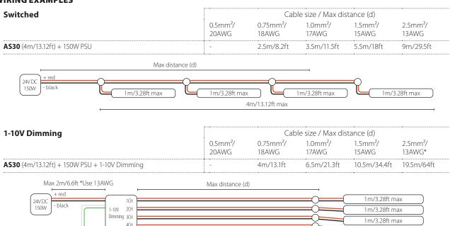
Note: This guide is produced from testing with KKDC approved power supplies or control gear.
